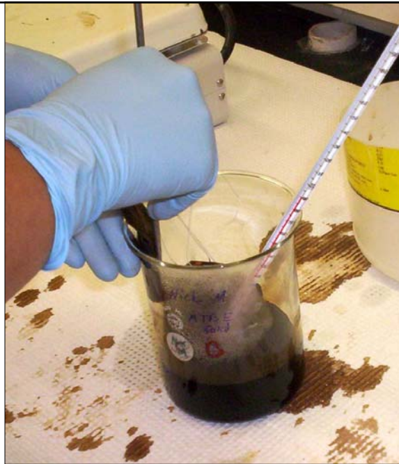
Using the spatula to squeeze tea bags against the side of the beaker
