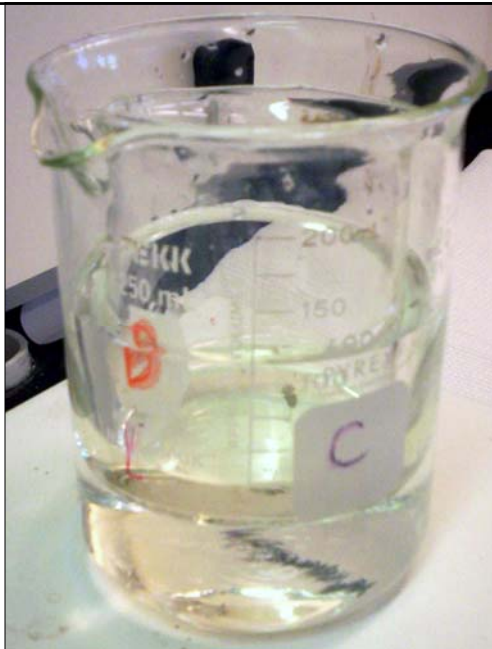
Beaker-within-a-beaker method of evaporating dichloromethane
