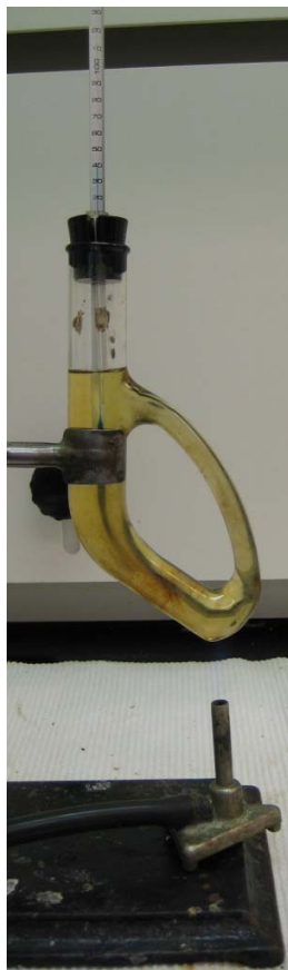
Figure 2: Thiele tube on stand with micro Bunsen burner.
