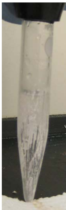
Figure 10: Extract on exterior of sublimation tube. The larger crystals have been scrapped into a beaker.
