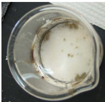
Figure 6: Water removed by \text{Na}_2\text{CO}_3 . Note the brown globules on the white surface.
