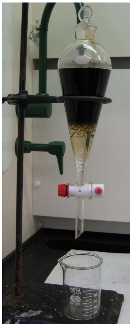
Figure 3: Separatory funnel with 30mL Dichloromethane and filtered tea. Note the emulsion at the boundary.
